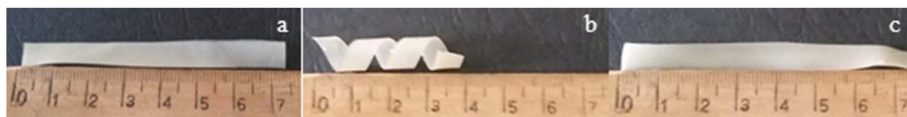
Figure 7. Illustration of the shape memory behavior for PU 7: (a) permanent, (b) temporary, (c) recovered shape. [Color figure can be viewed in the online issue, which is available at wileyonlinelibrary.com .]
